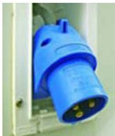
Connection to the mains is by means of a cable that can be plugged into the campervan exterior in the blue P17 socket. This socket includes a mandatory "earth" connection. Plug in the mains cable then activate the circuit breaker located next to the power pack, to provide power to the living area. To avoid damaging your charger, ensure that the supply provides 230V  $\pm 10\%$ .
